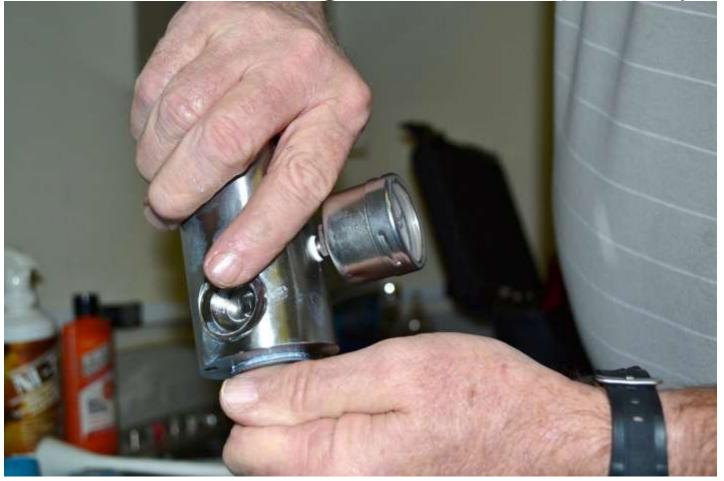
\* Be Careful To Keep The Pump In A Completely Vertical Position During Assembly.
