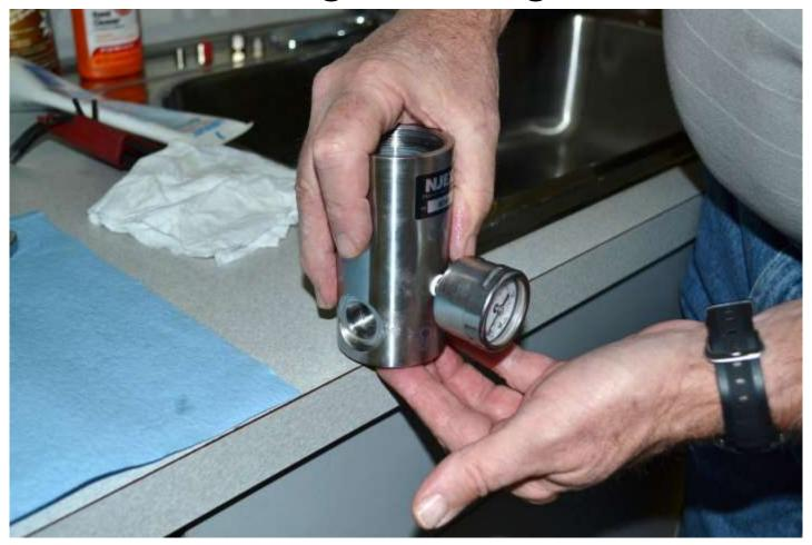
Screw Cartridge into Pump Body
