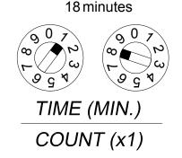
NOTE: The time (18 minutes) above corresponds to the dial setting shown for the Z65 model with the timer range setting in the factory position (jumper on the two left pins). See section 12.4 Timer Range Setting.
