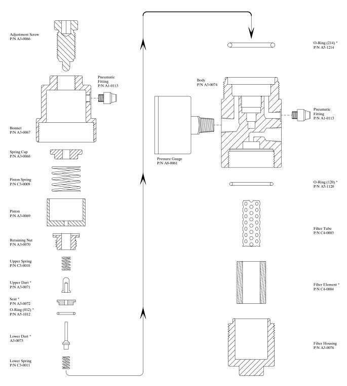
\* Filter/Regulator Repair Kit P/N D3-0003
