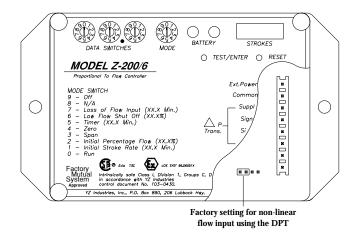
**B. Linear:** when using flow computer type flow inputs that are linear with respect to flow, the configuration jumper should be in the middle position marked linear.
