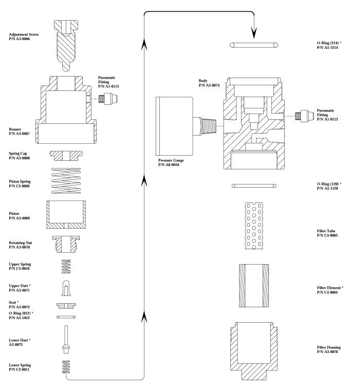
\* Filter/Regulator Repair Kit P/N D3-0003
