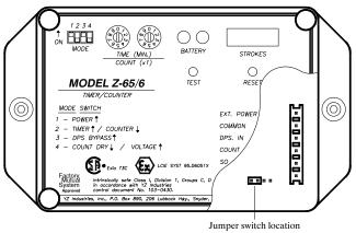
Jumper switch location for 1 - 99 counts (xx) factory positioned
