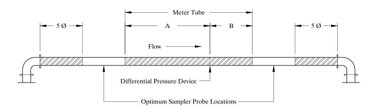
A = The number of unobstructed, straight pipe diameters upstream (see AGA - 3 manual). B = The number of unobstructed, straight pipe diameters downstream (see AGA - 3 manual).
