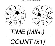
NOTE: The time (18 minutes) above corresponds to the dial setting shown for the Z65 model with the timer range setting in the factory position (jumper on the two left pins). See section 12.4 Timer Range Setting.
