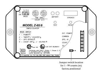
ON BEEE  $\circ$ STROKES  $\bigcirc$ TEST **MODEL Z-65/6** RESE TIMER/COUNTER  $\bigcirc$  $\bigcirc$ MODE SWITCH ] = 0 = 0 = 0 = 0 = 0 = C EXT. POWER - POWER T - TIMER ↑ / COUNTER ↓ COMMON DPS. IN - COUNT DRY↓ / VOLTAGE ↑ COUNT Exia 13C Ex LCIE SYST 95.D6051X 8 **8** 8 Intrinsically safe Class I, Division in accordance with YZ Industries
