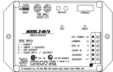
2. Dry Contact Input: mode switch 4 should be in the off position. Depress the test switch and hold. A red LED should illuminate. When the dry contact input is received at the counter input (ter. #3) the green LED will turn on and off and the red LED will illuminate again. This will normally occur very quickly and give the appearance that the green LED blinks on when the pulse input is received and removed.
