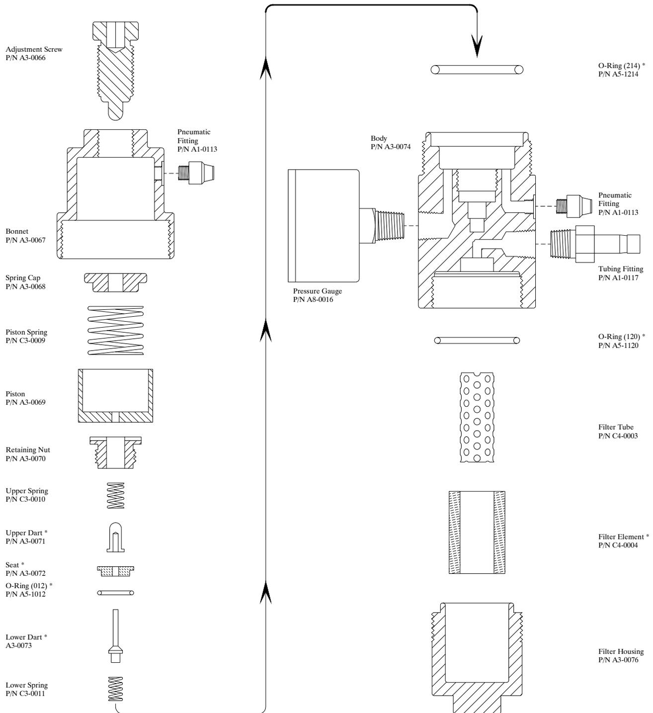
\* Filter/Regulator Repair Kit P/N D3-0003
