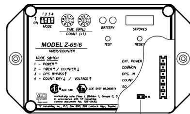
Jumper switch location for 1-99 counts (xs) factory positioned
