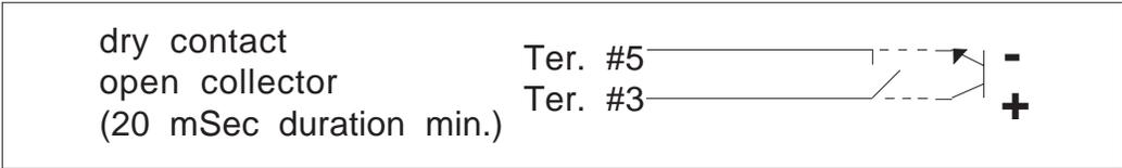
3. Voltage Pulse Input: move mode switch 4 to the on position. Depress the test switch and hold. A green LED should illuminate. When the voltage pulse input is received at the count input (ter. #3) the red LED will turn on and off and the green LED will illuminate again. This will normally occur very quickly and give the appearance that the red LED blinks on when the pulse input is received and removed.
