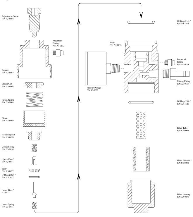
\* Filter/Regulator Repair Kit P/N D3-0003
