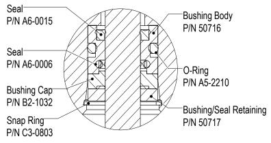
**Bushing Seal Assembly for Actuator Piston**
