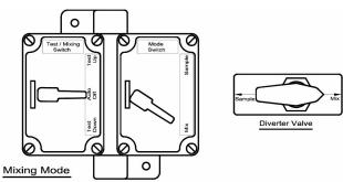
In the MIXING MODE, the Diverter Valve should be in the MIX position. Likewise, the mode switch should be in the MIX position. This will enable the Test / Mixing switch to be used as a mixing switch. In this position, the mixing rod and disc can be moved up and down through the product stored in the sample vessel to insure a homogeneous
