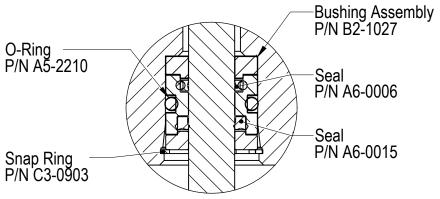
**Bushing Seal Assembly** for Precharge Inlet Head
