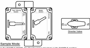
In the SAMPLE MODE, the Diverter Valve should be in the SAMPLE position. Likewise, the mode switch should be in the SAMPLE position. This will enable the Test / Mixing switch to be used as a test switch to verify proper operation of the sample pump.
