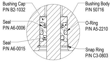
**Bushing Seal Assembly for Precharge Inlet Head**
