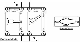
In the SAMPLE MODE, the Diverter Valve should be in the SAMPLE position. Likewise, the mode switch should be in the SAMPLE position. This will enable the Test / Mixing switch to be used as a test switch to verify proper operation of the sample pure.
