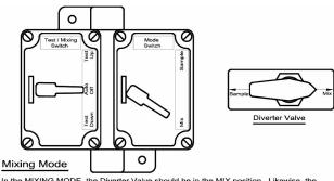
In the MIXING MODE, the Diverter Valve should be in the MIX position. Likewise, the mode switch should be in the MIX position. This will enable the Test / Mixing switch to be used as a mixing switch. In this position, the mixing rod and disc can be moved up and down through the product stored in the sample vessel to insure a homogeneous
