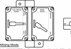
In the MIXING MODE, the Diverter Valve should be in the MIX position. Likewise, the mode switch should be in the MIX position. This will enable the Test / Mixing switch to be used as a mixing switch. In this position, the mixing rod and disc can be moved up and down through the product stored in the sample vessel to insure a homogeneous mixture.
