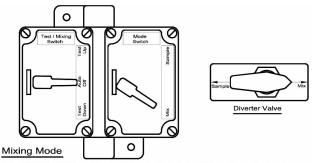
In the MIXING MODE, the Diverter Valve should be in the MIX position. Likewise, the mode switch should be in the MIX position. This will enable the Test / Mixing switch to be used as a mixing switch. In this position, the mixing rod and disc can be moved up and down through the product stored in the sample vessel to insure a homogeneous mixture.
