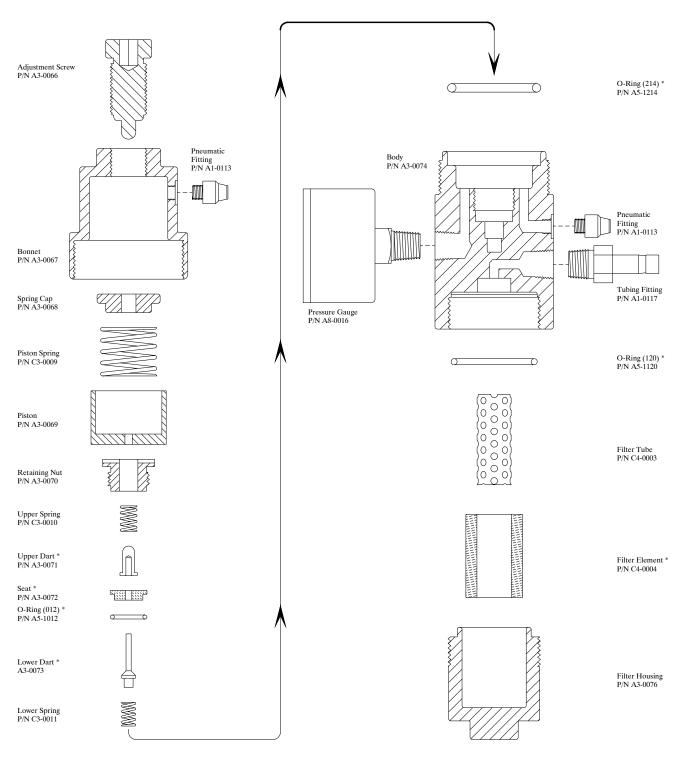
\* Filter/Regulator Repair Kit P/N D3-0003
