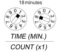
NOTE: The time (18 minutes) above corresponds to the dial setting shown for the Z65 model with the timer range setting in the factory position (jumper on the two left pins). See section 12.4 Timer Range Setting.
