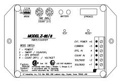
1. Dry Contact Input: mode switch 4 should be in the off position. Depress the test switch and hold. A red LED should illuminate. When the dry contact input is received at the counter input (ter. #3) the green LED will turn on and off and the red LED will illuminate again. This will normally occur very quickly and give the appearance that the green LED blinks on when the pulse input is received and removed.
