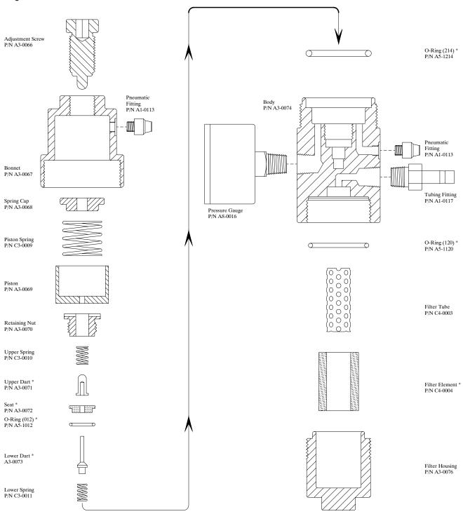
\* Filter/Regulator Repair Kit P/N D3-0003
