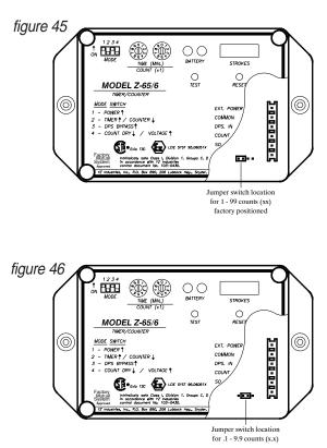
2. Z-65/6.03 Range Setting: x.x minutes: **set** the configuration jumper to the far left position (factory setting), figure 47.
