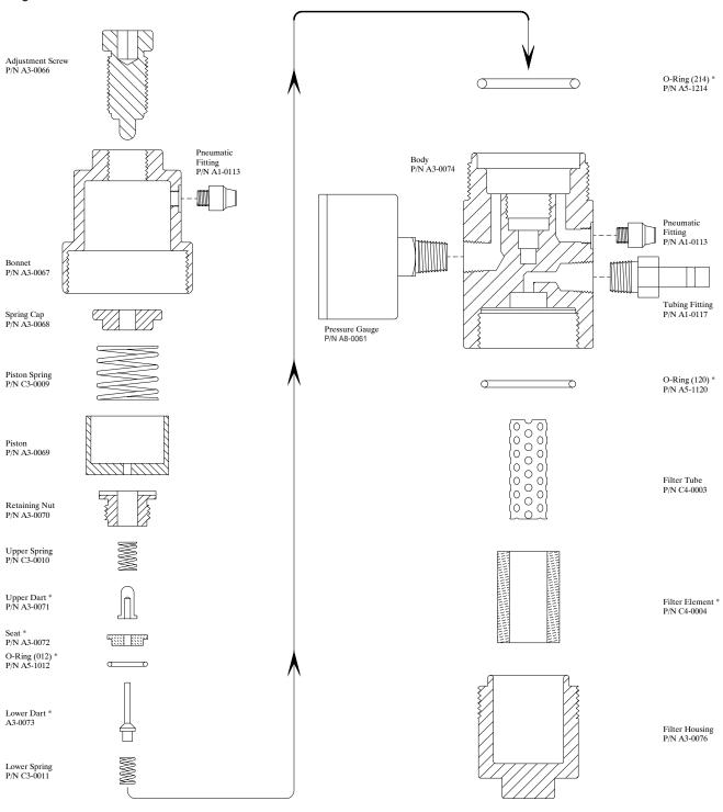
\* Filter/Regulator Repair Kit P/N D3-0003
