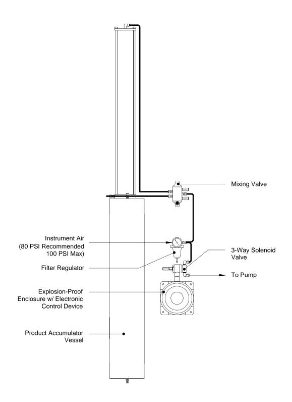
Electrical Wiring, Pneumatic -1A
