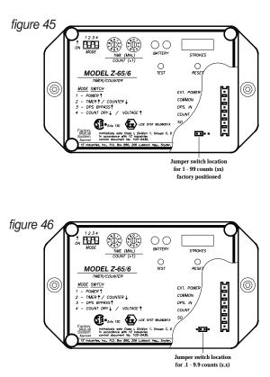
2. Z-65/6.03 Range Setting: x.x minutes: **set** the configuration jumper to the far left position (factory setting), figure 47.
